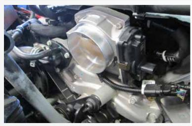
Now install BBK throttle body using supplied hardware and using 5mm wrench. Then reconnect plugs and factory air box back onto vehicle.
