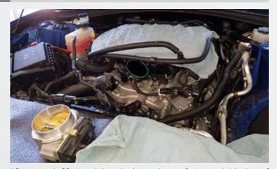
After removal of factory air-box check to make sure factory gasket is clean of debris.
