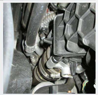
Start by loosening factory coupler clamp using 7mm socket do not remove.
