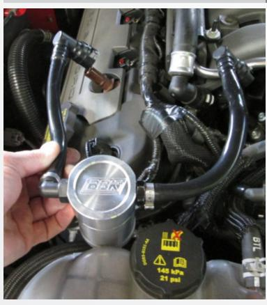
Install the (2) vacuum hoses supplied in the kit onto the BBK oil separator canister.
