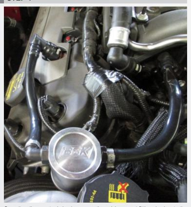
Once the oil separator is in place press the quick connect fittings back onto the barb fitting on the intake and valve cover.
