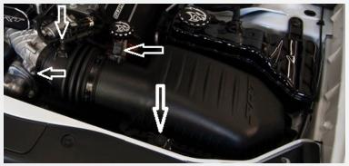
Unclip wiring from the mass air sensor, remove the vacuum tube from the inlet tube, loosen the clamp on the inlet tube, remove the bolt from the air box that connects it to the body.
