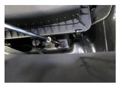
Remove the 10mm bolt on the right side of the air box that mounts it to the inner fender. Detach the air box from the lower inlet tube on the side of the radiator as you remove the air box. By pulling upwards and towards the firewall.
