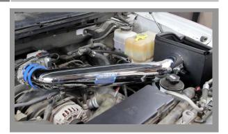
Install the blue BBK Coupler and BBK Intake Tube to the throttle body.
