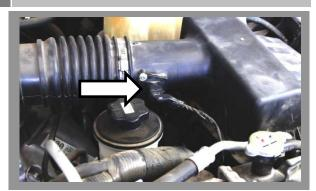
Disconnect the Mass Air Flow (MAF) Sensor.
