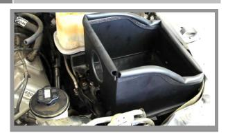
Place the cold air shield into the vehicle on the bottom half of the factory air box and use the three original clamps to secure the shield.
