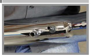
Install the supplied rubber grommet and straight fitting into the BBK Cold Air Tube.
