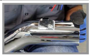
Remove the MAF Sensor from the stock intake system using a T-20 Torx and install it into the BBK Cold Air Tube using the supplied hardware. <u>NOTE!!!</u> The Air Flow of the sensor needs to be going towards the throttle body, the sensor should only fit one way because of the stagger in the hole pattern.
