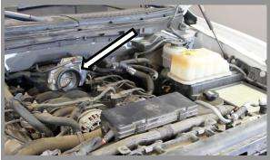
Unclip the three clips at the air box and remove the entire system out of the vehicle.
