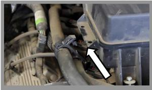
Loosen the two 10mm mounting bolts that secure the factory intake system to the vehicle.
