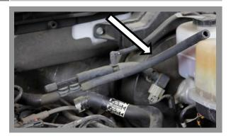
Remove the factory vent hose and replace it with the supplied 3/8" hose. Connect the supplied 3/8" hose to the plastic straight fitting on the BBK Intake Tube. The Valve Cover vent hose with the clip will be connected to the larger welded tube coming off the BBK Intake Tube.
