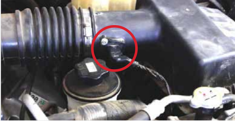
Disconnect the Mass Air Flow (MAF) Sensor.
