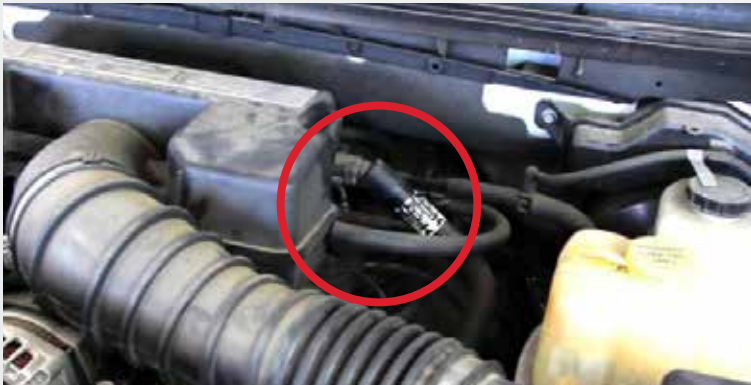
Remove the two vent hoses going into the factory intake system.
