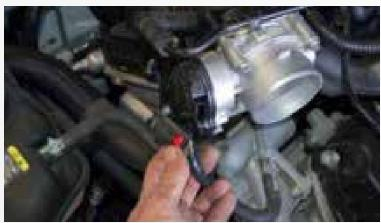
Unplug the electrical connector from the side cover of the throttle body. Pull the black wire harness mount out of the hole in the throttle body.
