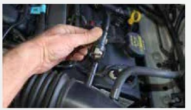
Disconnect the (2) breather hoses attached to the inlet tube
