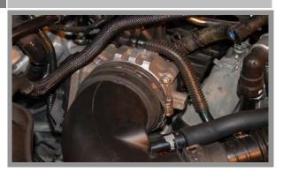
Re-install the air inlet tube and reconnect the breather tube. A little WD-40 or light grease on the inside of the tube may help in this process. Tighten Clamps.
