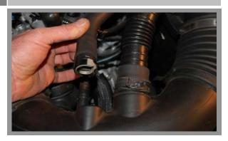
Disconnect the smaller plastic breather tube from the air inlet tube. You can leave the sound tube connected.
