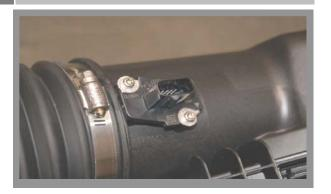
Remove the Mass Air Sensor from the stock air box tube. Install in the aluminum mounting base on the BBK inlet tube with the 2 supplied 4mm
