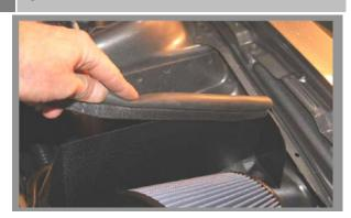
Install the supplied sponge seal to the top of the air filter shield and trim off any excess
