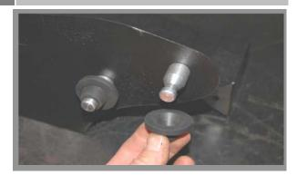
Assemble the 2 aluminum pins to the bottom of the BBK air filter shield using the supplied ¼-20x ½" Philips screws. Install the stock rubber grommets onto the pins.
