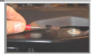
Remove the plastic radiator cover by prying up the center of the plastic pin heads at the slots cut on each side. Pull the pins out to remove. Lift cover and set aside.
