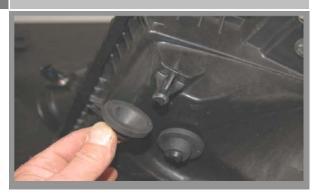
Remove the bolt on the right side of the stock air box that mounts it to the inner fender. Detach the air box from the lower inlet tube on the side of the radiator as you lift the box out to remove. Detach the Mass Air Sensor wire harness from the side of the air box by slightly pulling on the harness at each barbed mounting pin. Remove the 2 rubber grommets from the bottom of the air box.
