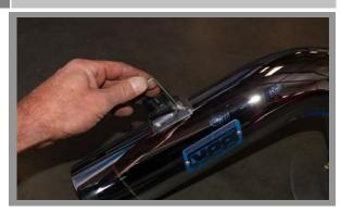
Install Mass Air sensor into the BBK inlet tube at the aluminum mount. Use the supplied Allen screws.
