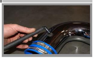
Install the supplied grommet in the bottom of the chrome inlet tube for the breather hose. Install the black plastic 90 degree fitting into the supplied 3/8" hose and push other end of Fitting into grommet. Install blue connector and clamps onto throttle body side of the tube.
