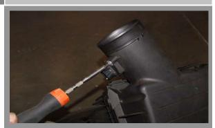
• Using a Torx T20 bit, remove the Mass Air Sensor.
