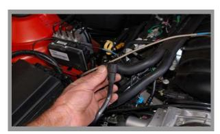
Loosen clamp on air inlet tube at throttle body. Disconnect plastic breather hose from tube at passenger side valve cover. Remove two nuts that secure the air box. Remove inlet tube and air box.
