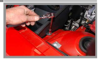
Install the spongy trimming on the top of the shield and the rubber trimming in the hole the cold air tube will go through. Drop the filter shield into place lining up the aluminum pin with the stock rubber mounting grommet. Install shield over stock mounting stud and use stock nut to retain.
