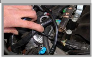
Route breather hose straight back under the throttle body and away from the idler pulley. Connect the hose to the steel breather line you disconnected the stock one from.
