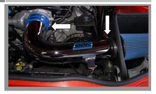
Set the filter into the filter shield and install the chrome inlet tube into the hole in the shield and onto the throttle body. Position filter on the end of the inlet tube. The filter clamp should be on the engine side of the filter shield. Tighten clamps at throttle body and filter.
