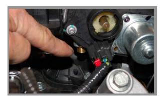
With your digital volt meter, recheck the voltage on the top wire. If the voltage is not the same as your first reading, then turn the brass adjuster stud to adjust the voltage reading until it is. Turn the ignition key to the OFF position. Disconnect the negative battery terminal.
