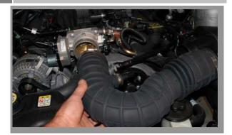
Disconnect the breather tube from the air intake tube. Loosen the clamps at the throttle body and at the air box then remove the air intake tube.
