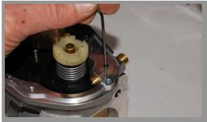
With a 2.5mm allen wrench, loosen the set screw for the brass adjuster stud.
