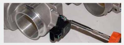
Remove the TPS sensor and re-install on the BBK Throttle Body using the stock screws.
