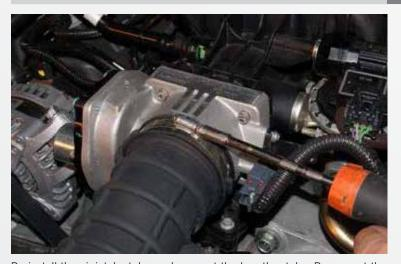
Re-install the air intake tube and connect the breather tube. Reconnect the negative battery terminal.
