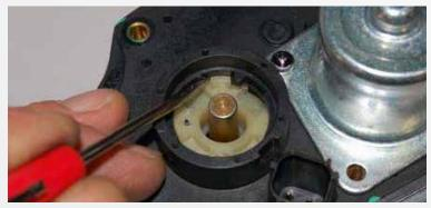
Pop off the round plastic cover on the motor cover. Install the cover on the throttle body. Using a small screwdriver, push the white spring retainer down while rotating it 160 degrees counter clockwise until the large and small tabs align with their slots. Release and allow the tabs to seat.
