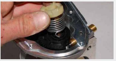
Install the internal spring on the gear in the BBK Throttle Body. Make sure the hook on the end of the spring is in its mounting hole in the gear.
