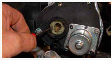
Using your small screwdriver, push in on the white spring retainer to release the spring. Unplug and remove the motor cover. Tighten the set screw for the brass adjuster stud. Reinstall the motor cover, reclock the internal spring counter-clockwise and lock the tabs into place. Reinstall the round plastic cover. Plug in the motor control wires.
