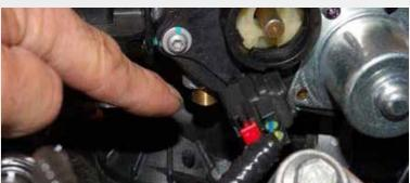
With your digital volt meter, recheck the voltage on the top wire. If the voltage is not the same as your first reading, then turn the brass adjuster stud to adjust the voltage reading until it is. Turn the ignition key to the OFF position. Disconnect the negative battery terminal.
