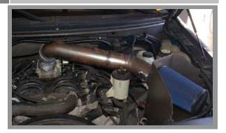
Install the chrome inlet tube into the hole in the filter shield then on to the connector on the throttle body. Rotate the inlet tube for the best position and tighten the clamps at the blue connector. Install the filter on to the end of the inlet tube and tighten the clamp.
