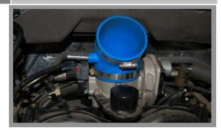
Install the blue connector and two clamps onto the throttle body.
