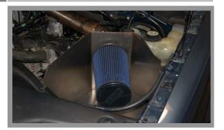
Install the BBK filter shield on the driver side inner fender. Use supplied bolts and washers to mount the shield.
