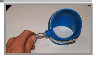
Install the provided 3/8" diameter by 2" long aluminum adapter tube. Push the long end into the port on the side of the provided blue hose connector. This is the new breather tube connection point.
