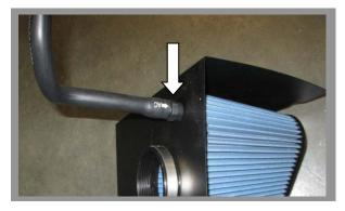
The 6.1L Engines require the use of the straight fitting for the breather hose.
