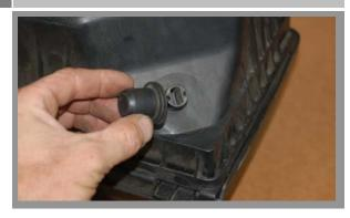
On the bottom rear of the stock air box, remove the rubber grommet for re-use with the BBK filter shield.
