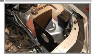
Place the filter shield into place in the engine compartment and line up the grommet with its hole. Mount the front tab of the filter shield using the stock bolt.
