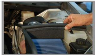
From the supplied hardware kit, find the aluminum pin and 1/4" Phillips screw and install on the BBK filter shield. Install the stock rubber grommet onto the pin. Install the supplied sponge rubber seal to the top of the filter shield.
