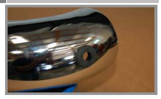
From the hardware kit, install the supplied rubber grommet into the hole in the BBK Inlet Tube. Install the Air Temperature Sensor into the grommet.
