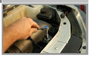
Remove the bolt that mounts the front of the air box to the vehicle. Lift out the air box and remove with the inlet hose.
