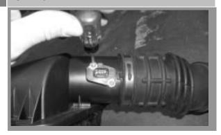
Remove the 2 torx screws from the mass air meter and slide the meter out of the stock inlet hose, and then install it into the BBK inlet pipe using the supplied screws.
