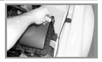
Loosen the hose clamp that attaches the inlet hose to the throttle body. Remove the bolt that holds the air filter box to the driver side fenderwell.
