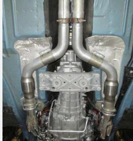
Now after headers are installed install supplied head pipe assembly the driver side and passenger side are labeled with little stickers on exhaust.
