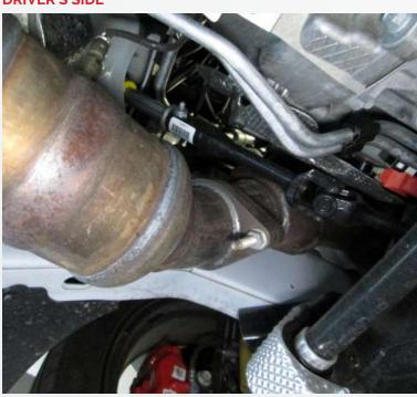
Disconnect  $O^2$  sensor plugs and then remove factory head pipe using 16mm socket.
