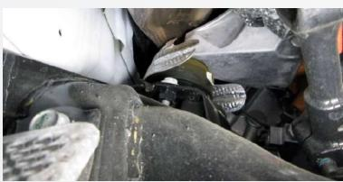
Start removing the 18mm nuts on motor mount at frame them remove 15mm bolts attached to from motor mount to engine and remove. At this time raise engine at least 1 inch for extra room. Then with 10mm socket/wrenches remove factory heat shield and manifold. Make sure at this time to check for any carbon build up on cylinder head and clean for flat sealing surface.
