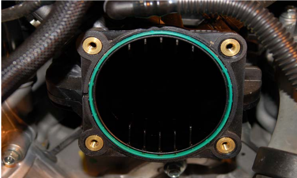
Fig. 5 Reuse the stock O-ring style gasket. Just wipe off oil and debris with a rag.
