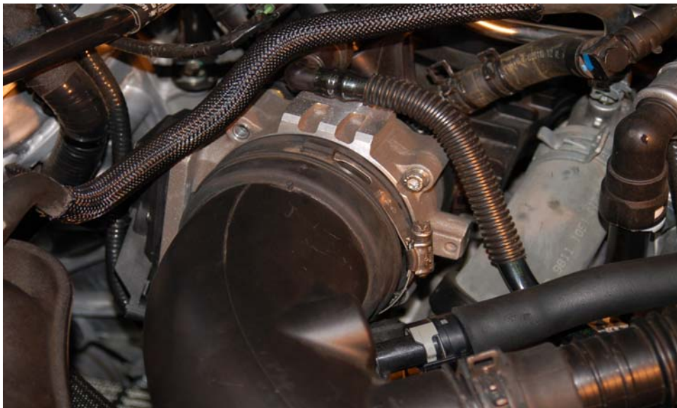
Fig. 6 BBK Throttle Body shown installed. Stock air inlet tube will fit the 85mm opening.
