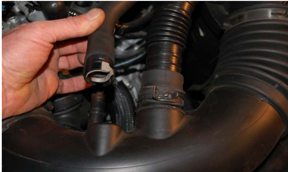
Fig. 2 Remove smaller breather tube. Larger sound tube can stay connected.
