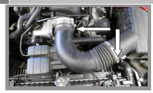
• Loosen the clamps at the throttle body and factory air box.
