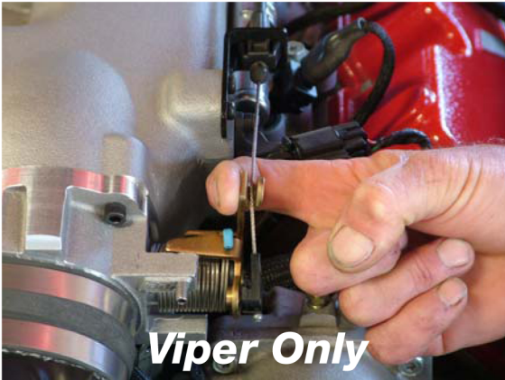
Slightly bend bracket by hand to align cable
