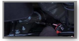
• Starting on the driver side, loosen the clamps at the mufflers and mid pipes.
