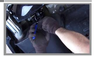
• Using a pry bar or grommet removal tool, remove the rubber grommet located by the muffler tip from the muffler hanger.
