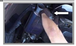
• Slide the muffler over the inlet pipe, then slide the grommet closest to the rear bumper onto the muffler hanger.
