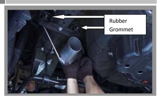
• Starting on the driver side, slide the inlet pipe through the 2 hanger grommets and into the mid pipe and snug the clamp to hold the tubing in place.
