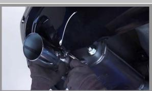
Slide and snug the exhaust tip onto the outlet tube of the muffler. STEP 12
