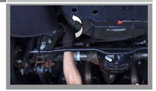
• Twist the mid pipe so the muffler has enough clearance to be removed.
