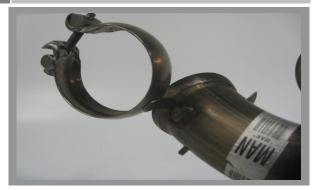
NOTE!! On 2011-2013 Models you will need to remove the factory clamp from the stock muffler to use on the inlet tube for the BBK Axle Back System. The clamp has a very small and brittle tack weld on it only for the factory production line use. Its easily removed by cutting or wiggling the clamp back and forth until it breaks off the stock muffler.
