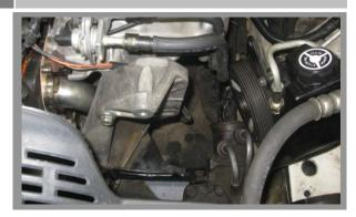
After removing the belt and un-mounting the steering pump, move it off to the side to aid in Header installation.
