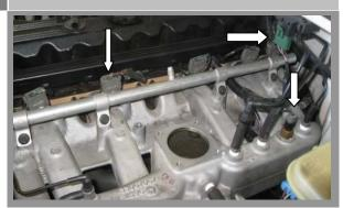
Disconnect all the fuel injector connections (6 total) and any other electrical connections for the intake manifold.
