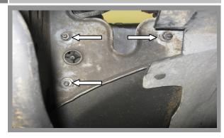
• From underneath the vehicle remove the 3 nuts that secure the stock air box assembly.
