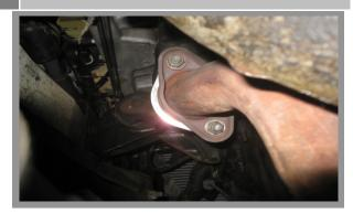
While still underneath the vehicle, remove the hardware from the collector to the head pipe.
