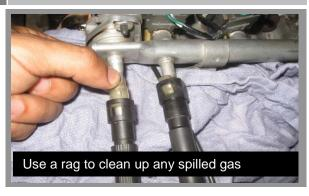
Be sure there is no pressure in the fuel system and disconnect the 2 fuel lines going to the fuel rails by squeezing the tabs and pulling back on the lines.
