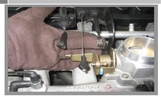
Unclip the cable attachments from the throttle body linkage.
