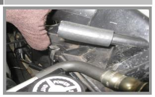
Remove the clips holding the top half of the stock air box assembly together to the bottom half, and also remove both vent hoses going to the air box.
