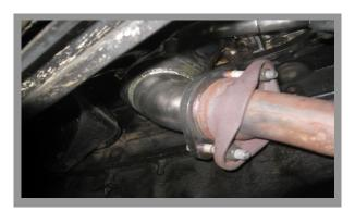
Re-install the Air Intake Assembly and tighten the header to the head pipe using the supplied hardware.
