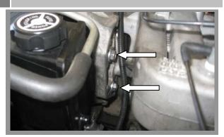
Remove the 2 mounting bolts on the back of the steering pump.
