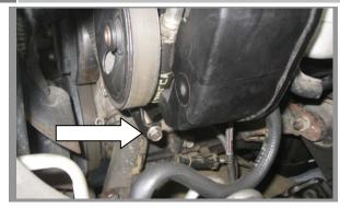
Remove the long adjusting bolt from underneath the steering pump.
