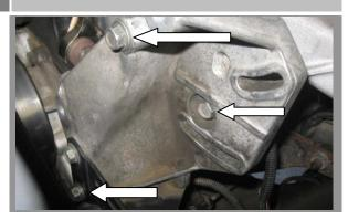
Remove the 3 bolts holding the steering pump bracket to the intake manifold.
