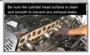
Place the BBK Header into position and tighten the header down using the stock hardware.
