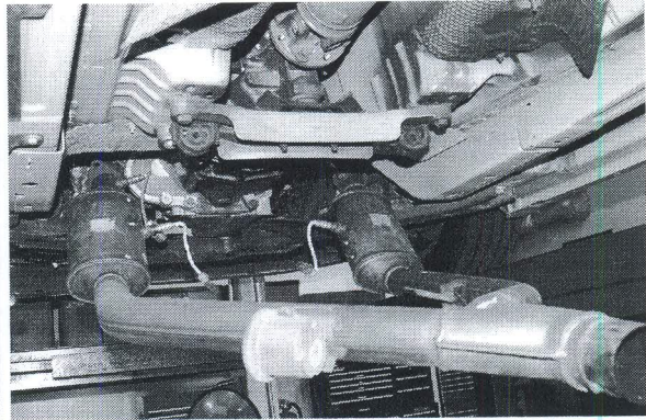
FIG. 2 Remove nuts at exhaust manifolds and drop midpipe out
