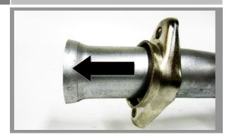
• Slide the flared flanges over the head pipes so that the flared end of the flanges match the flared end of the head pipes as shown.
