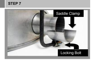
• Use the hanger and saddle clamp for the outlet of the muffler. Slide the hanger through the corresponding rubber grommet on the chassis then snug the hanger into the saddle clamp and tighten the locking bolt to hold the hanger in place.
