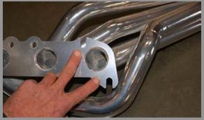
Remove the studs that correspond to the notches in the BBK Header flange. You will install supplied bolts in these spots. <u>NOTES!!!</u> There are 2 thread pitches supplied. Because the manufacturer changed the thread pitch used after 2011 you will have to compare the supplied bolt to the factory stud to confirm which thread pitch to use.
