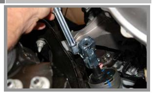
• Remove the 2 bolts from the steering U joint at the rack and pinion, remove the U-joint so the shaft can hang out of the way.
