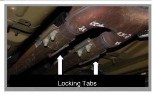
Separate the cat-back system by loosening the (2) 15mm nuts on each band clamp and prying the locking tabs up with a small flat head screwdriver while sliding the clamp towards the rear of the car.
