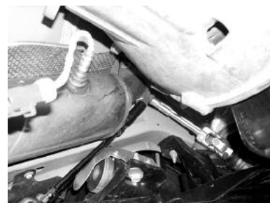
Unbolt from exhaust manifolds
