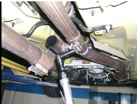
Separate H-pipe from tail pipes
