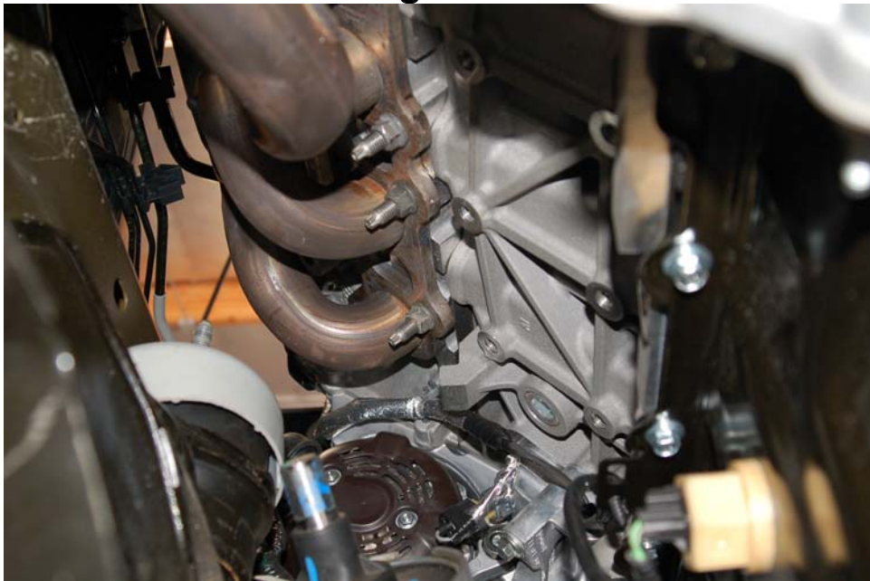
Motor mount removed.
