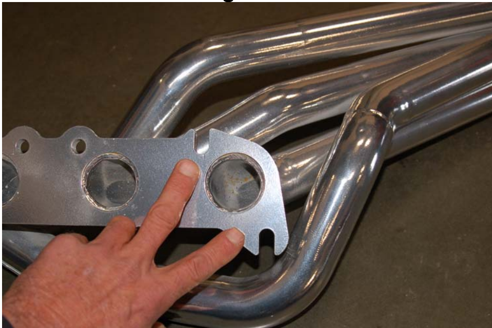
Remove stock studs that correspond with notches in flange. Use supplied bolts.
