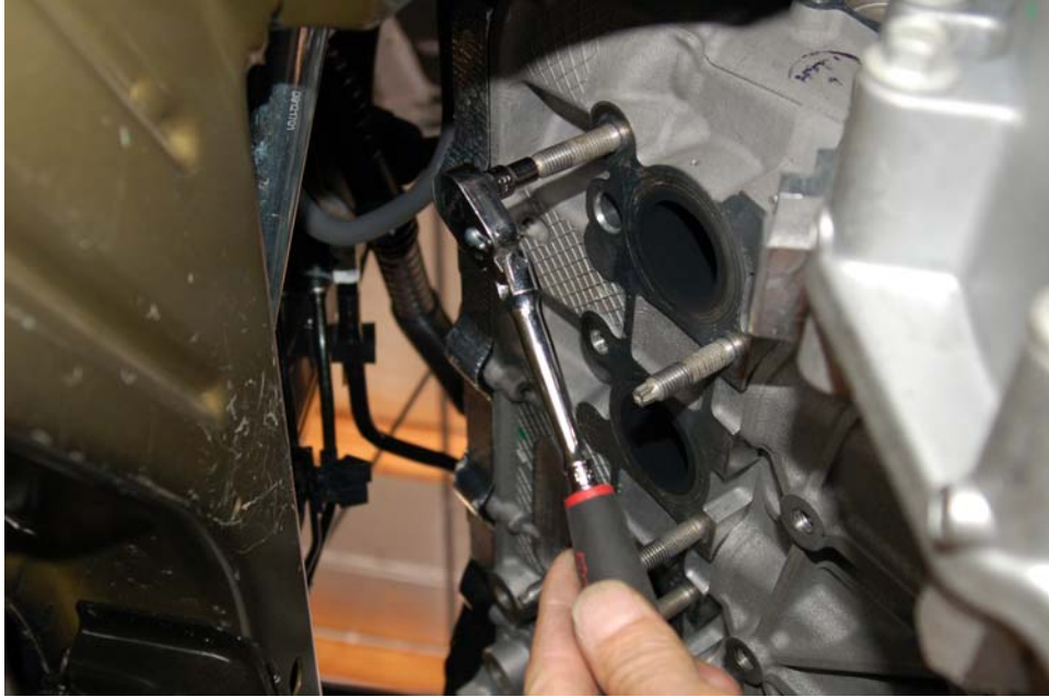
Removing stock studs.
