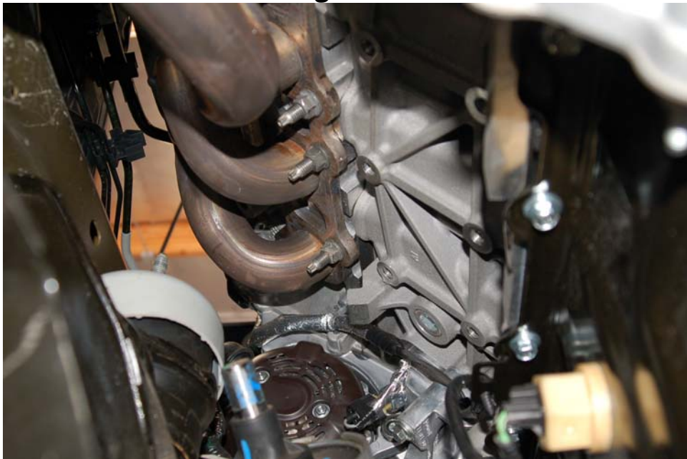
Motor mount removed.
