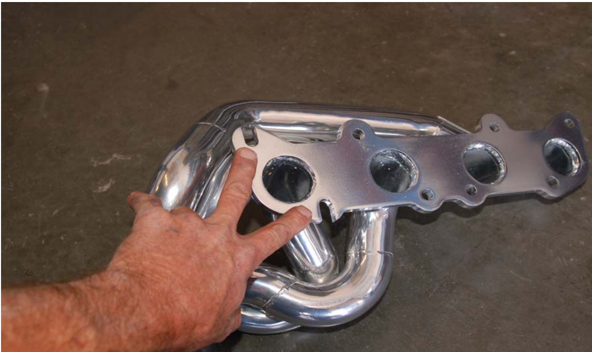
Fig.2 Shows notches where bolts will be installed and studs removed.
