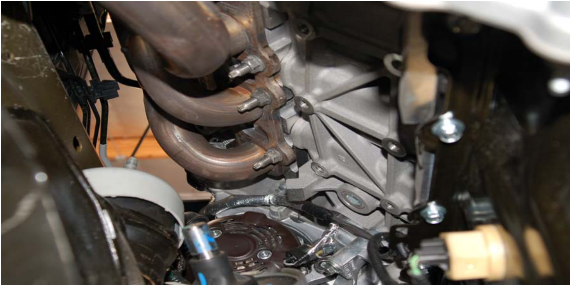
Fig 1. Motor Mount removed. Shows nut access.
