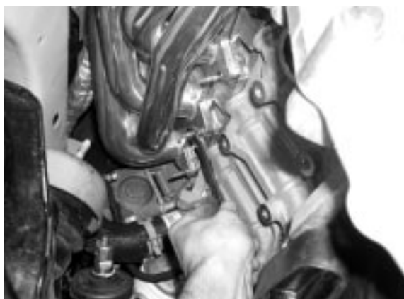
Remove dipstick tube.
