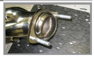
Install the supplied studs onto the BBK Header Collectors.
