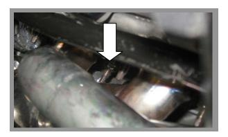
For both the driver side and passenger side place the supplied BBK Gasket and header into place. Then Tighten. <u>NOTE!!!</u> The passenger side is a little more tricky. Make sure to leave all the nuts loose so the header has room to move. With the stock x-pipe hanging out of the way, the bottom rear nut needs to be tightened from behind the collector.
