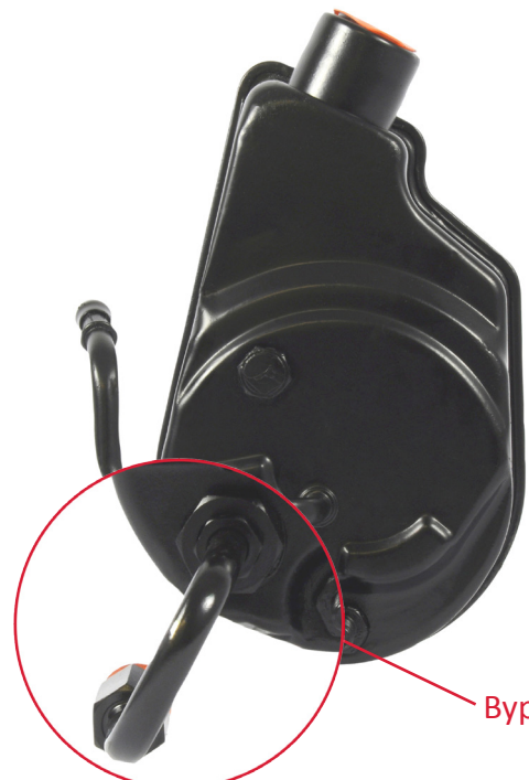
Pump with Bypass Pipe Installed
