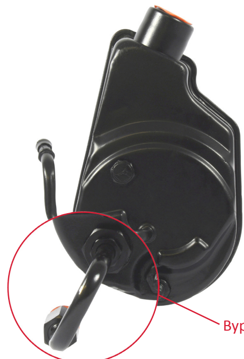
Pump with Bypass Pipe Installed
