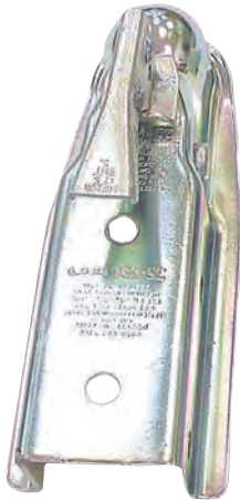
Fulton coupler after 336 hours salt spray testing.
