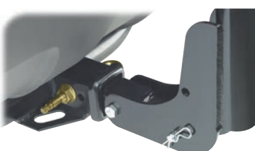
Tighten nut on J-Pin shaft, compressing ball mount or hitch-mounted accessory against receiver tube
