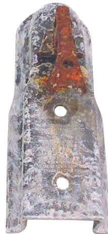
Competitor's coupler after 336 hours salt spray testing.
