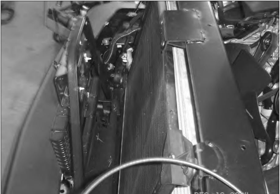
Figure 13 Latch support moved out of the way
