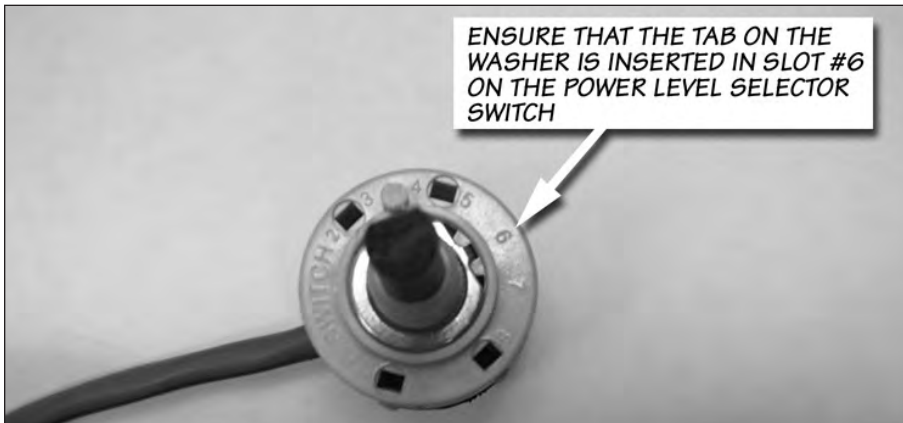
Figure 49: Finished installation of the Power Level Selector Switch on 2003-04 model year vehicles
