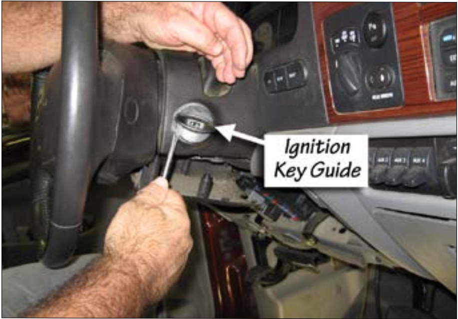
Figure 20 Remove Plastic Ignition Key Guide
