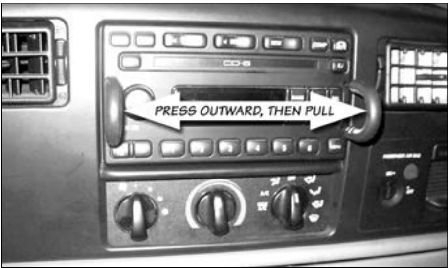
Figure 23: Removal of the stereo (03-04 model year vehicles only)
