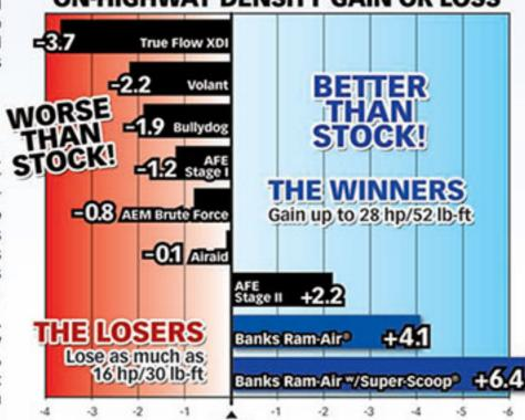
Testing performed on a 2004 Dodge Ram 2500 4x4, Quad Cab, Long Bed with 325 HP engine. Data taken at 2800 RPM in 3rd gear under full power conditions on a 6% grade. Total weight of truck & trailer = 21,650 lbs.
