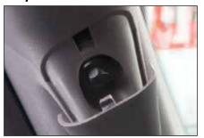
**2.** Remove stock pillar by pulling towards you and sliding up, releasing the two tabs from the dash. Disconnect speaker wire harness to fully remove stock pillar. See **Step 2**.
