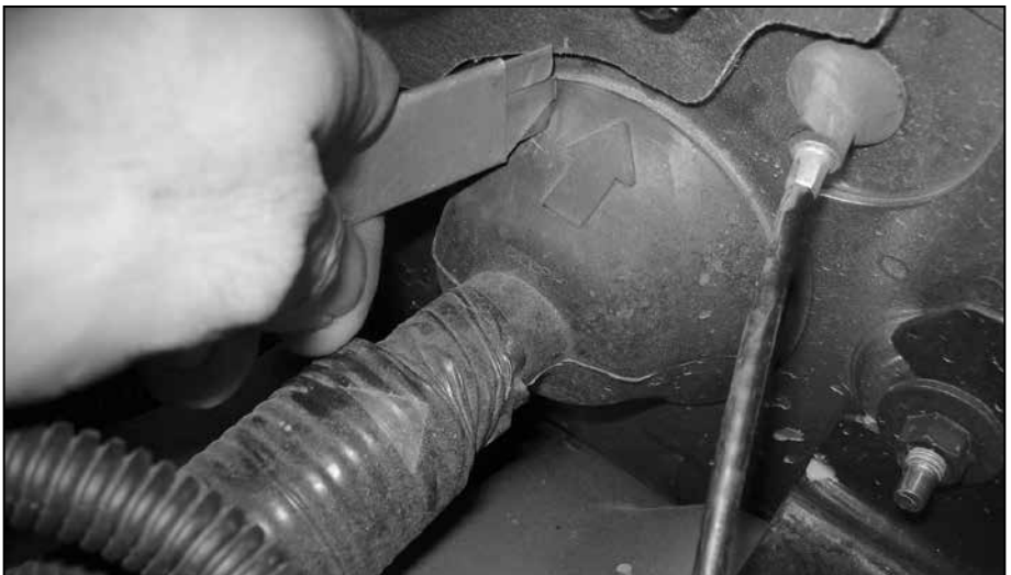
Figure 5 Driver Side Firewall, Rubber Grommet
