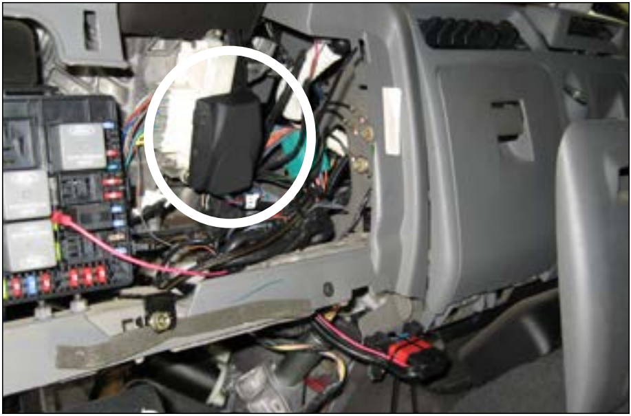
Figure 23 SpeedBrake Module Mounting Location
