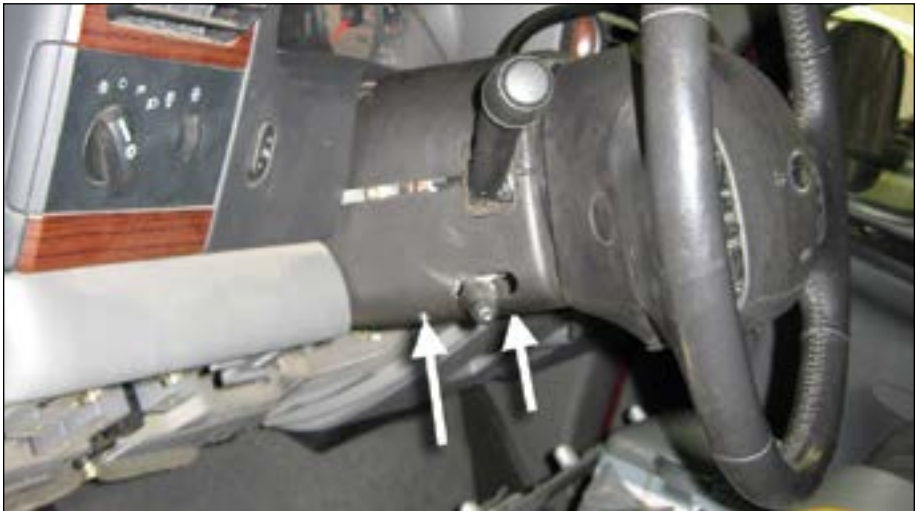
Figure 20 Remove column panel covers
