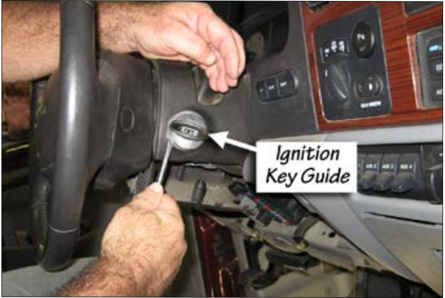
Figure 21 Remove Plastic Ignition Key Guide
