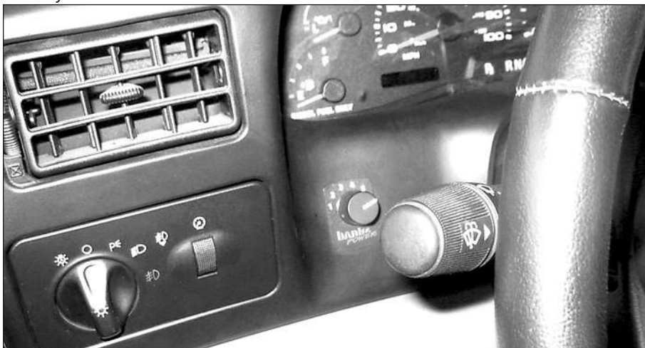
Figure 51: Finished installation of the Power Level Selector Switch on 2005-07 model year vehicles
