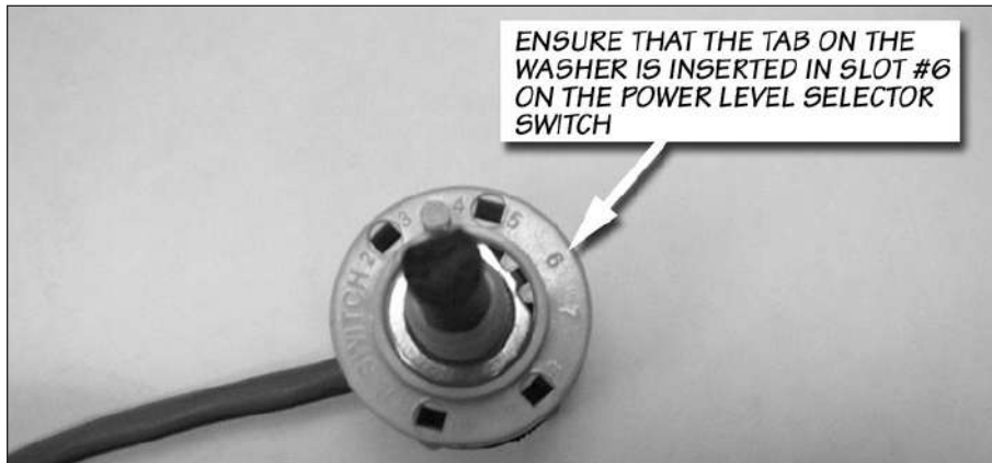
Figure 50: Finished installation of the Power Level Selector Switch on 2003-04 model year vehicles
