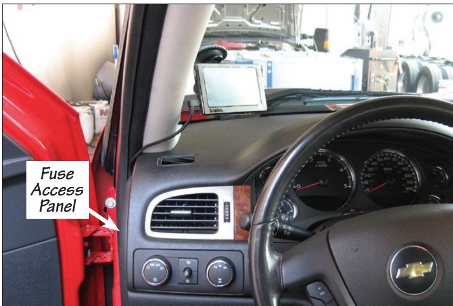
Figure 40 Mounting location for Banks iQ, Chevy LMM Shown
