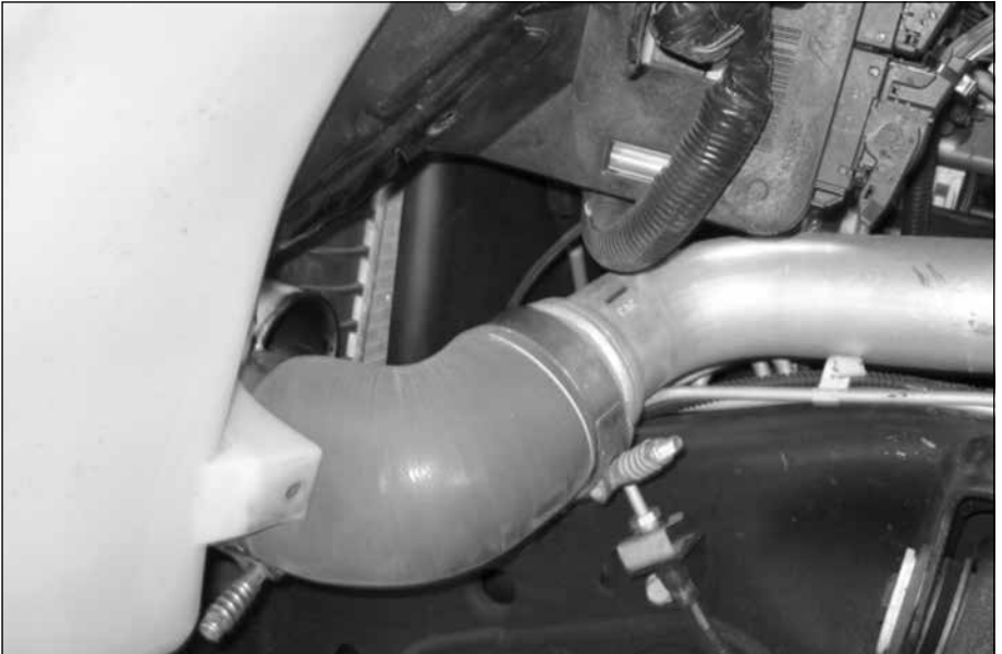
Figure 17 Drivers side boost hose
