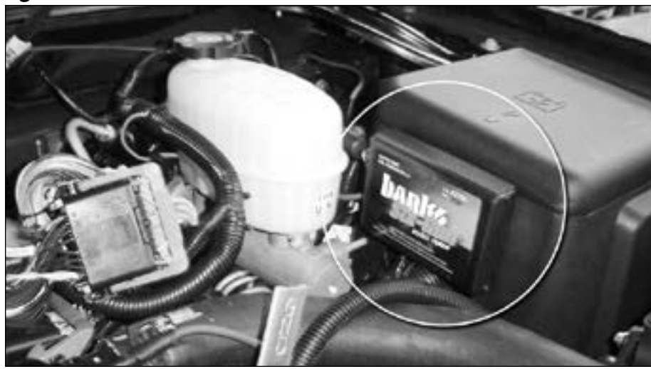
Figure 4 Six-Gun module mounted on fusebox
