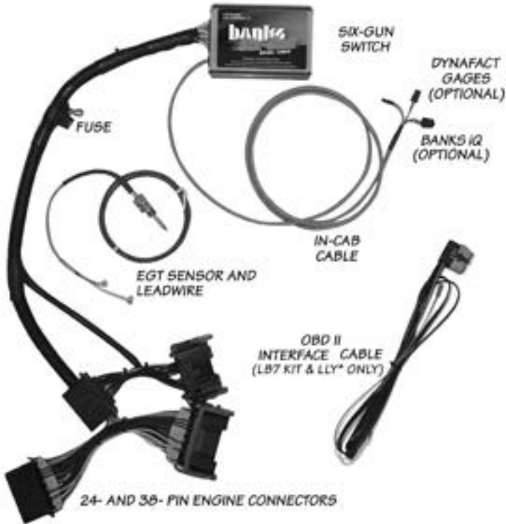
Figure 1 Six-Gun and supplied wiring harness
