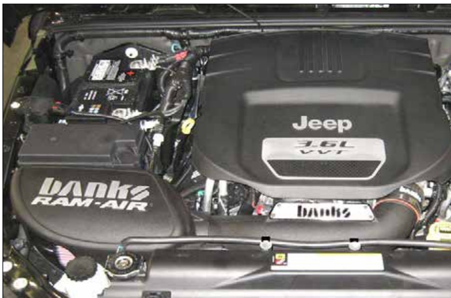
Figure 8- Installed Banks Ram-Air Intake System
