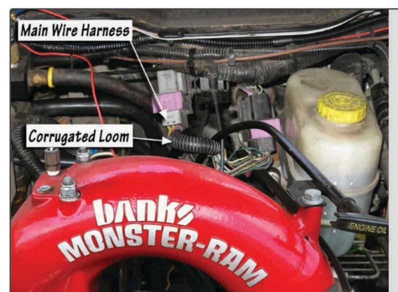
**NOTE:** For 2004-2007 model vehicles, locate the supplied corrugated loom in your kit and install over the main connector wires to protect it from rubbing against the dipstick.
