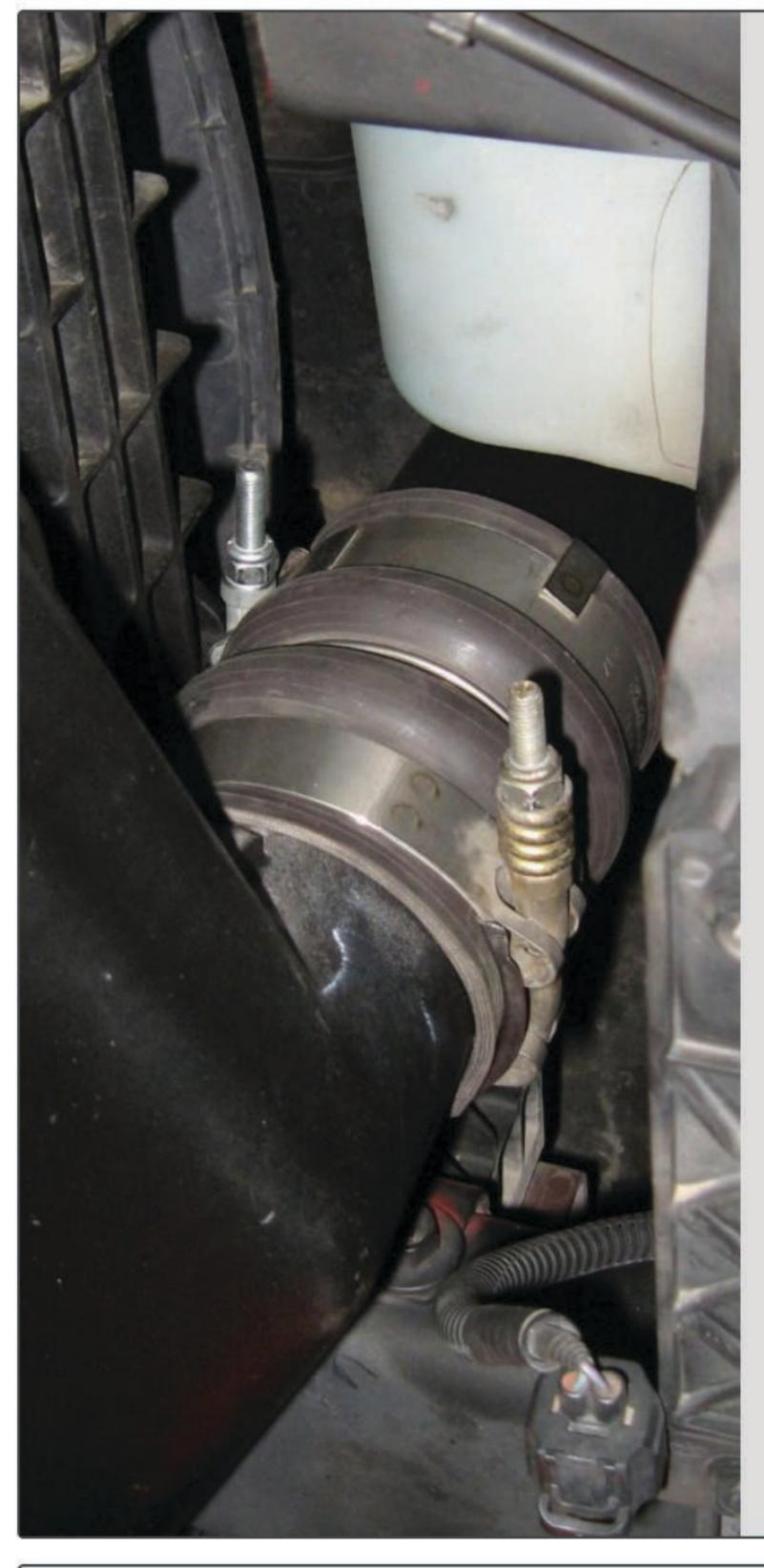
1. Install Banks driver-side boost tube. The driver-side tube uses a 3.5-inch diameter hump hose and spring-loaded clamps at the connection to the Banks Monster-Ram and re-use the factory hose and clamps at the CAC. Keep the hose clamps loose until the Monster-Ram is installed. The orientation of the hose clamps should be position as shown here to avoid clearance issues. Cover the opening of the boost tube to prevent foreign objects from entering the boost tube during the installation.
